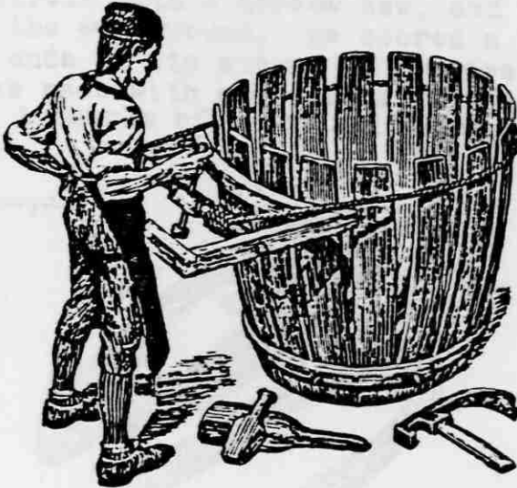
Assembling a big barrel with the simpler kind of cooper's windlass
